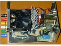
Before I begin, what was I using before? Here are two pictures of my previous station power supply. This consisted of an ex-COMPAQ PC 300W PSU repackaged in an aluminium box with connectors on the front panel.
